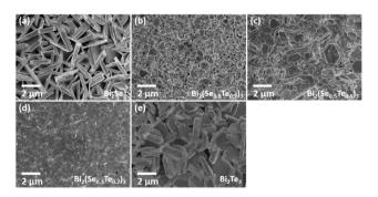
Fig. 3 SEM images showing the morphologies of the Bi<sub>2</sub>Se<sub>3</sub> (a), Bi<sub>2</sub>Te<sub>3</sub> (e) and ternary Bi<sub>2</sub>(Se<sub>1-x</sub>Te<sub>x</sub>)<sub>3</sub> (b–d) films deposited by LPCVD under similar conditions (550 °C/0.05 mmHg) onto SiO<sub>2</sub>-coated silicon substrates.
