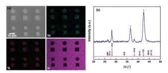
Fig. 1 (a) SEM image with EDX mapping and (b) grazing incidence XRD pattern from  $Sb_2Te_3$  selectively deposited from  $[SbCl_3(Te^nBu_2)_3]$  into 30 μm TiN holes and an indexed bulk pattern of Sb<sub>2</sub>Te<sub>3</sub>. <sup>42</sup> The TiN substrate peaks are marked by \*.
