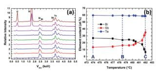
Fig. 6 (a) EDX spectra and (b) relationship between  $(Bi_{1-y}Sb_y)_2Te_3$  film composition and the increasing temperature of deposition (indicating the temperatures at positions A, B and C).
