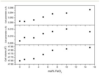
Fig. 5 Variation of cell parameters a, c and cell volume of the films with a change of mol% FeCl $_3$  added to the precursor solution. The increase of cell parameters confirms the incorporation of Cl into the ZnO lattice.
