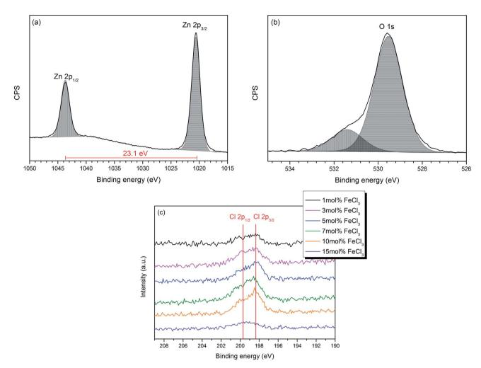
Fig. 3 High-resolution XPS spectra of (a) Zn 2p<sub>3/2</sub> (b) O 1s of the Cl-doped ZnO film formed from 10 mol% FeCl<sub>3</sub> and (c) Cl 2p for all films.
