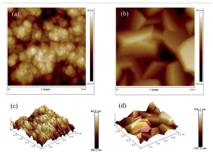
Fig. 7 AFM images of (a) undoped ZnO and (b) 10 mol% FeCl<sub>3</sub> doped ZnO and 3D images of the same area (c) and (d).
