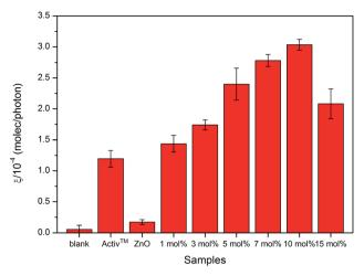
Fig. 8 The formal quantum efficiency (FQE) for the degradation of stearic acid on undoped and Cl-doped ZnO films under UVA illumination. Pilkington Activ glass is used as reference. All ZnO:Cl films are photocatalytically active and 10 mol% FeCl<sub>3</sub> added show the best efficiency.
