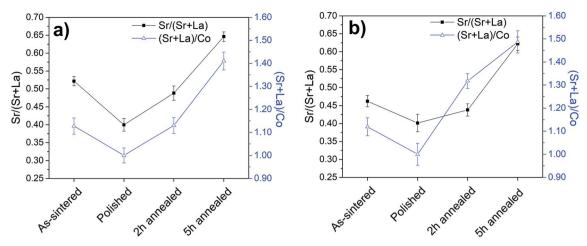
Fig. 4 Surface chemistry of LSC64 pellets characterized by (a) nano-probe AES and (b) XPS. The quantification shown from AES refers only to the particle free-regions of the LSC64 pellet surface.
