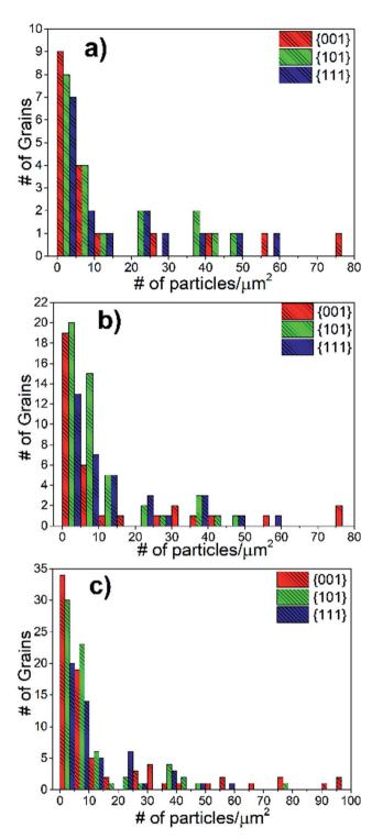
Fig. 8 The total distribution of precipitate number density on differently oriented grains at the surface of LSC64 pellets annealed at 800 °C for 2 h and 5 h. The grain orientations were processed with (a) 10°, (b) 15° and (c) 17.5° tolerance angles from the major orientations.
