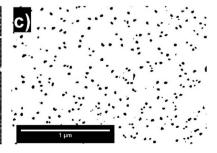
Fig. 7 (a) SEM secondary electron image of an area within a grain having some precipitates. (b) The same SEM image as in (a), with improved contrast upon applying the FFT filter. (c) The same SEM image as in (b), after performing background subtraction. The number density and area coverage of precipitates were calculated on the images after background subtraction.
