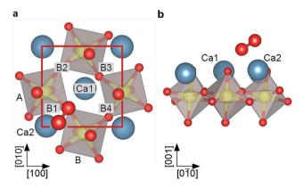
Fig. 2 DFT model of  $O_2^-$  adsorbed on  $Ca_3Ru_2O_7$ . (a) Top view and (b) side view of the vdW-DFT model for  $O_2^-$  with  $E_{ads}=1.4$  eV. The molecule adsorbs as a tilted superoxo species close to a Ca-Ca bridge (here B1)
