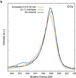
Fig. 8 Surface spectroscopies. (a) Point Kelvin probe spectroscopy of the pristine surface and the (2  $\times$  1)  ${\rm O_2}^-$  overlayer at 78 K. Shown are the measured (full line) and the numerically fitted (dashed lines) Kelvin parabolas, reflecting a change in work function (see main text for analysis details). (b) O 1s XPS (Mg K $\alpha$ ,  $T_{sample}=110$  K) spectra of the ascleaved surface, the (2  $\times$  1)  ${\rm O_2}^-$  overlayer and after annealing at 210 K for 30 min.
