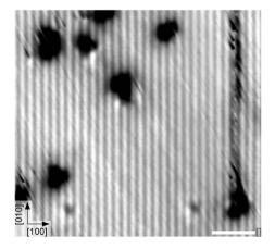
Fig. 4 STM image after dosing 0.025 L  $O_2$  at 110 K. The molecules appear as streaks across point defects. STM parameters:  $V_{\rm sample} = +1.0$  V,  $I_{\rm tunnel} = 0.1$  nA,  $T_{\rm sample} = 78$  K; fast scan direction is  $58^{\circ}$  clockwise from horizontal. The scale bar corresponds to 3 nm.
