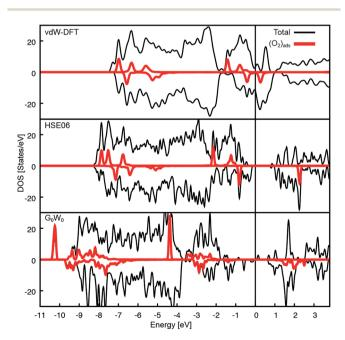
Fig. 6 Density of states for the (2  $\times$  1) overlayer. Total and O<sub>2</sub> DOS for the different theoretical approaches. In all cases charge is transferred into the split  $\pi^*$  states of the O<sub>2</sub> in the spin down channel. The HOMO–LUMO gap is 0.7, 3.1 and approximately 1.7 eV on the DFT, HSE06 (insulating phase) and G<sub>0</sub>W<sub>0</sub> level, respectively.
