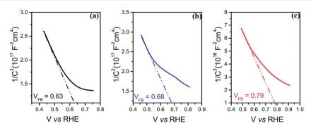
Mott-Schottky measurements of (a) p-Si/TiO<sub>2</sub> (b) p-Si/TiO<sub>2</sub>/CoO<sub>x</sub> and (c) p-Si/TiO<sub>2</sub>/NiO<sub>x</sub>.
