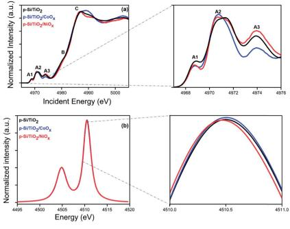
Fig. 7 X-ray spectroscopy characterization of p-Si/TiO<sub>2</sub> (black), p-Si/TiO<sub>2</sub>/CoO<sub> $_X$ </sub> (blue), p-Si/TiO<sub>2</sub>/NiO<sub> $_X$ </sub> (red): (a) HERFD-XANES spectra acquired at the Ti K-edge. The magnified view on the right shows the pre-edge peaks. (b) Kα emission lines. The magnified view on the right shows the Kα peak maximum.
