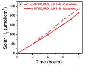
Fig. 8 Photo-electrochemical performance of the p-Si/TiO $_2$ /NiO $_x$  photoelectrode recorded under 1 sun illumination in artificial seawater at pH 8.4 (red) or pH 7.0 (black; 0.2 M phosphate buffer): (a) linear sweep voltammograms, (b) photo-current density measured at -0.3 V<sub>RHE</sub> and (c) comparison of calculated (open squares) and measured (closed squares) photo generated hydrogen per geometric surface area of the photo-electrode at -0.3 V<sub>RHE</sub> and 1 sun.
