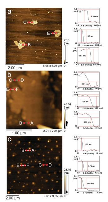
Fig. 3 AFM topographical images (left) and the respective height curves (right) of the samples GR-BZ (a), GR-BZ/HX (b) and GR-HX (c).
