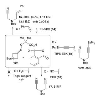
Scheme 5 Extension to other C-C bond forming reactions. Reaction conditions: 5 mol% 4c, K2CO3 (1.1 equiv.), 0.05 M DCE, blue LEDs, rt, 1 h. <sup>a</sup>Reaction run of reagent 16 (2 equiv.) for 14 h. NMR vield is given (isolated yield: 31%) breaction run of reagent 18 (2 equiv.) for 24 h.
