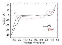
Fig. 6 Cyclic (CV) and square wave (SWV) voltammograms of 1 (1 mM) in THF (internal standard Fc/Fc\*,  $v = 0.1 \text{ V s}^{-1}$ ).
