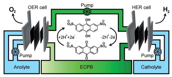
Fig. 1 The concept of ECPB-assisted water splitting in a dual electrolyser setup. The OER cell on the left oxidises water whilst reducing the ECPB. The reduced ECPB is then transported to the HER cell, where it is re-oxidised with concomitant  $H_2$  production. The gas evolution reactions can now be separated in time and space, mitigating the issues of gas crossover during water electrolysis.
