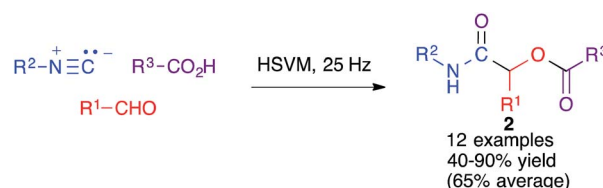
Scheme 2 The mechanochemical Passerini reaction.
