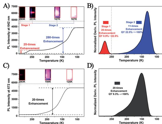
Fig. 6 The PL intensity at the fixed points of (A) 642 nm for the Ag<sub>29</sub>(BDT)<sub>12</sub>(TPP)<sub>4</sub> NC and (C) 672 nm for the Pt<sub>1</sub>Ag<sub>28</sub>(S-Adm)<sub>18</sub>(TPP)<sub>4</sub> NC at different temperatures. Insets: the digital photographs of each NC in DMF solution under UV light. The derivative results for PL intensity of (B) Ag<sub>29</sub>(BDT)<sub>12</sub>(TPP)<sub>4</sub> and (D) Pt<sub>1</sub>Ag<sub>28</sub>(S-Adm)<sub>18</sub>(TPP)<sub>4</sub> NCs.
