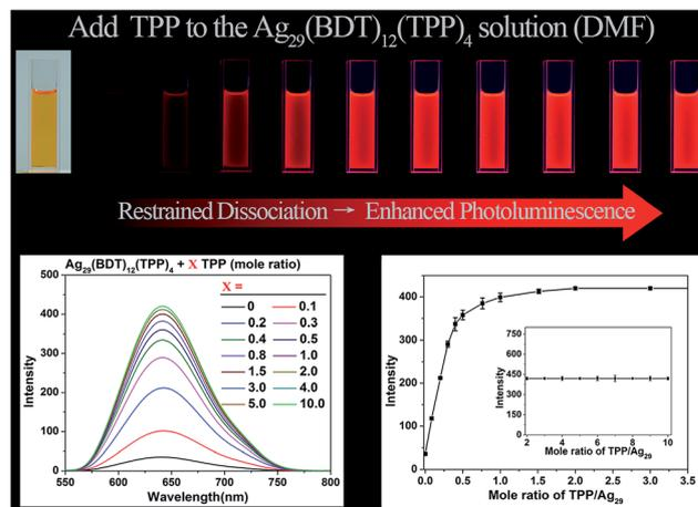
Fig. 4 PL variation trend of the  $\text{Ag}_{29}(\text{BDT})_{12}(\text{TPP})_4$  NC resulting from the addition of different molar ratios of TPP ligand. (Top) PL intensity variation monitored by digital photography of the  $\text{Ag}_{29}(\text{BDT})_{12}(\text{TPP})_4$  NC in the solution state under UV light. (Bottom-left) PL intensity variation monitored using the fluorescence spectrometer. (Bottom-right) PL intensity variation monitored at the fixed point of 642 nm.
