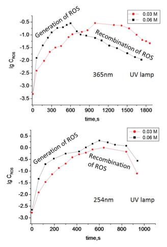
Fig. 3 Log concentration of ROS generated in TiO<sub>2</sub> suspensions of different concentration (0.03 M and 0.06 M) under irradiation by UV light with different wavelengths vs. irradiation time.
