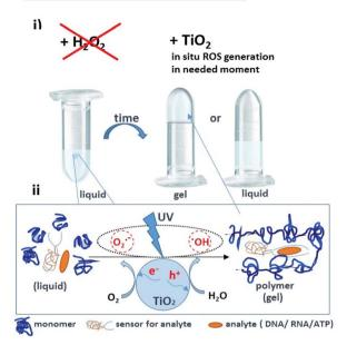
Fig. 1 (i) A portable sensor based on a light-induced liquid-to-gel transition for polymer by radical polymerization on  ${\rm TiO_2}$  particles. The details of the sensor design are shown in Fig. 5; (ii) ROS formation on titania *via* reactions with photogenerated photohole (h<sup>+</sup>) and photoelectron (e<sup>-</sup>).
