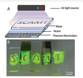
Fig. 7 (A) Scheme of photolithography process (negative resist) by radical polymerization of acrylamide initiated by ROS generated on  ${\rm TiO_2}$  anodized surface (TNT) under UV light 365 nm; (B) experiment of polymerization of test-sample on TNT allows further test improvement.
