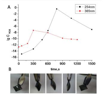
Fig. 6 (A) Log concentration of ROS generated on  ${\rm TiO_2}$  nanotubes (TNT) under UV irradiation at different wavelengths vs. time. (B) Radical polymerization of acrylamide initiated by ROS generated on TNT under UV irradiation at 365 nm.
