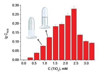
Fig. 4 The dependence of the log concentration of ROS generated on  ${\rm TiO_2}$  particles on  ${\rm TiO_2}$  suspension concentration. Inserts show the minimum concentration of  ${\rm TiO_2}$  particles in a suspension (therefore minimum concentration of ROS generated on  ${\rm TiO_2}$  particles), needed for the gel formation.
