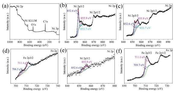
Fig. 7 XPS survey spectrum and the Ni 2p and Fe 2p core-level XPS spectra obtained from (a and b) the pristine surface and (c and d) worn surface of the G-Ni-3 sample, and (e and f) worn surface of the steel ball.
