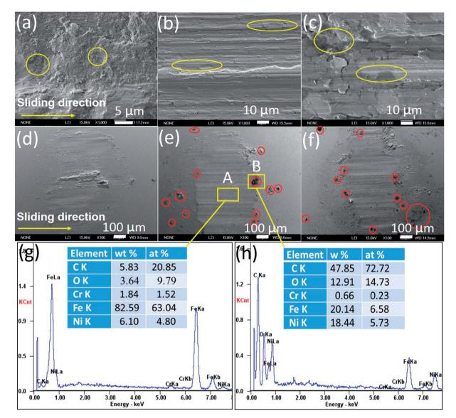
Fig. 6 SEM images (a–f) and EDS (g and h) of the worn surfaces of (a and d) pure Ni, (b and e) G-Ni-3 and (c and f) G-Ni-4 the samples and the pairing steel balls.
