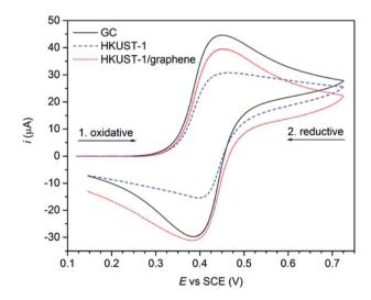
Fig. 7 CV measurements (recorded using a Ag/AgI reference electrode in  $0.01 \, M \, TBA \cdot BF_4$ /acetonitrile, sweep rate:  $0.1 \, V \, s^{-1}$ ) on a blank GC plate (black), a HKUST-1-covered GC plate (blue) and a composite film on GC (red) using 2 mM Fc as redox probe. These curves were obtained applying baseline removal and iR compensation to the original voltammograms (see Fig. S13†).
