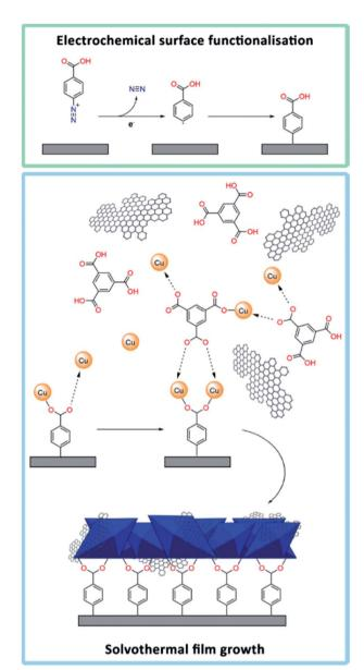
Fig. 1 Graphical representation of the HKUST-1/graphene film formation: (top) electrografting of 4-carboxyphenyl diazonium salt onto a GC substrate. (Bottom) solvothermal synthesis of an HKUST-1/graphene composite film, which is covalently tethered to the functionalised GC plate. The carboxylates on GC coordinate to  $\text{Cu}^{2+}$  (charges not shown) and thereby act as HKUST-1 nucleation sites. The graphene sheets, precursors, and HKUST-1 crystals (blue octahedra) are not shown on scale.
