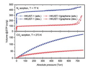
Fig. 5 (Top) Adsorption (filled symbols) and desorption (open symbols) curves at 77 K for  $\rm N_2$  over bulk HKUST-1 (blue) and over the composite (red). (Bottom) adsorption and desorption curves for  $\rm CO_2$  at 273 K of the same samples. The isotherms show higher adsorption capacity of the bare MOF compared to HKUST-1/graphene.
