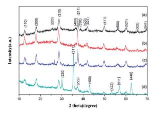
Fig. 3 X-ray diffraction patterns of (a) MnO<sub>2</sub>, (b) MnO<sub>2</sub>/PPy, (c) GO/ MnO<sub>2</sub>, (d) GMFP.
