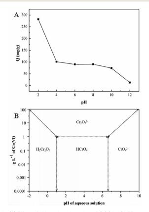
Fig. 5 (A) Effect of pH on the adsorption of Cr(vi) by GMFP: temperature, 298.15 K; adsorption time, 6 h; and initial Cr(vi) concentration, 300 mg  $L^{-1}$ , (B) relative distribution of Cr(vi) species in water as a function of pH and Cr(vi) concentration (adapted from ref. 1).
