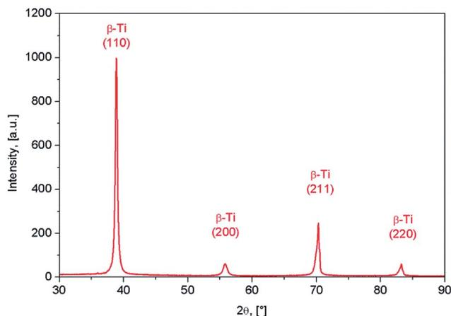
Fig. 2 XRD spectra of Ti-31.7Nb-6.21Zr-1.4Fe-0.16O (% wt) Gum-type alloy.
