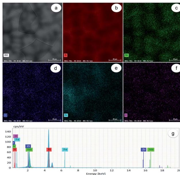
Fig. 1 Dispersion of alloying elements in Ti-31.7Nb-6.21Zr-1.4Fe-0.16O (% wt) Gum-type alloy microstructure: (a) SEM-BSE image of investigated field; (b) dispersion map of Ti; (c) dispersion map of Nb; (d) dispersion map of Zr; (e) dispersion map of Fe; (f) dispersion map of O; (g) EDS spectrum of investigated field. Scale bar:  $40 \mu\text{m}$ .
