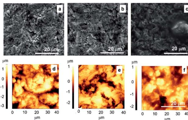
Fig. 5 SEM (a–c) and AFM (d–f) micrographs of the Gum alloy (a and d) functionalized with GNP (b and e), and GNP-SS (c and f) by MAPLE (266 nm, 600 mJ cm<sup>-2</sup>). The scanned area by AFM was 40 × 40 μm<sup>2</sup>. Scale bar: 20 μm.
