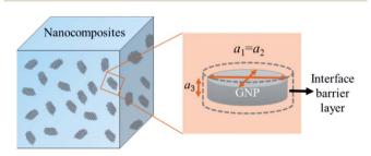
Fig. 2 Schematic for a composite unit of a GNP coated with a thin interfacial thermal barrier layer.
