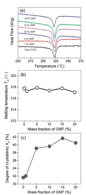
Fig. 5 (a) DSC curves of pure PTFE and GNP-PTFE nanocomposites. Melting temperature  $T_{\rm m}$  (b) and the degree of crystallinity  $X_{\rm c}$  (c) for pure PTFE and GNP-PTFE nanocomposites as a function of mass fraction of GNP.
