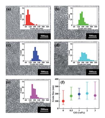
Fig. 2 SEM images of perovskite thin films (a) pristine, with (b) 0.5 vol%, (c) 1 vol%, (d) 2 vol%, and (e) 3 vol% GO in the perovskite precursor. The insert in each image shows the corresponding grain size distribution. (f) The average grain size as the function of GO amount.
