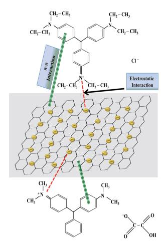
Fig. 6 A proposed mechanism for the adsorption of malachite green and ethyl violet on graphene oxide—gold nanocomposite by representing the possible interactions between dyes and graphene oxide—gold nanocomposite.
