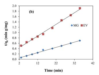
Fig. 5 Plots of (a) pseudo first-order kinetic medal, (b) pseudo second-order kinetic model for malachite green (MG) and ethyl violet (EV) adsorption. Reaction conditions; 7  $\mu$ M solution of each dye = 50 ml, 100 rpm, 30 °C.
