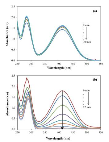
Fig. 7 UV-vis absorption spectra for the gradual reduction of 2-nitroaniline (a) in the absence of catalyst (b) in the presence of catalyst. Reaction conditions; 0.5 mM aqueous solution of 2-nitroaniline = 50 ml, NaBH $_4$  = 0.1 g, graphene oxide–gold catalyst = 5 mg, 30 °C, 100 rpm.
