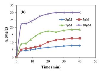
Fig. 3 Effect of initial concentration of dyes on the adsorbed amount of (a) malachite green and (b) ethyl violet on graphene oxide–gold nanocomposite. Reaction conditions; adsorbent =  $0.005 \, \text{g}$ , volume of dyes solution =  $50 \, \text{ml}$ ,  $100 \, \text{rpm}$ ,  $25 \, ^{\circ}\text{C}$ .
