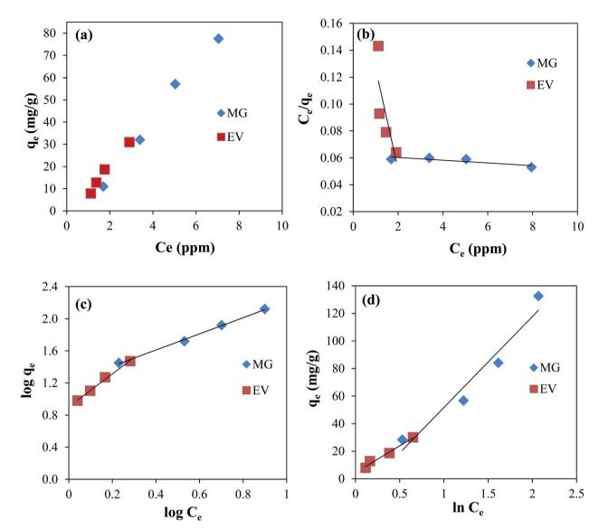
Fig. 4 Plots of (a)  $q_e$  verses  $C_e$ , (b) Langmuir isotherm, (c) Freundlich isotherm, and (d) Temkin isotherm for the adsorption of MG and EV dyes on GO–Au nanocomposite. Reaction conditions; adsorbent = 0.005 g, concentration of dyes solution = 3, 5, 7, and 10  $\mu$ M volume of dyes solution = 50 ml, 100 rpm, 25 °C.
