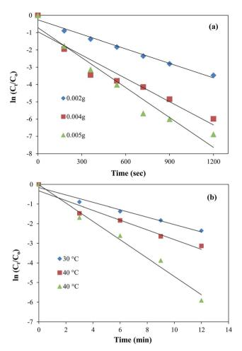
Fig. 8 Dependence of  $k_{\rm app}$  on (a) the amount of catalyst at 30 °C and (b) temperature. Reaction conditions; 0.5 mM aqueous solution of 2-nitroaniline = 50 ml, NaBH<sub>4</sub> = 0.1 g, graphene oxide–gold catalyst = 5 mg, 100 rpm.
