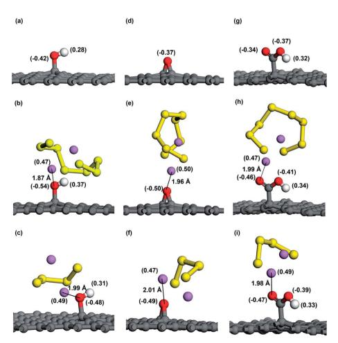
Fig. 5 Mulliken charge distribution before and after adsorption of  $\text{Li}_2\text{S}_8$  and  $\text{Li}_2\text{S}_4$  of (a–c) hG, (d–f) eG and (g–i) cG respectively. Note that charge of each atom is shown in parentheses. The shortest distance between Li atom and O atom is also shown in angstroms (Å).
