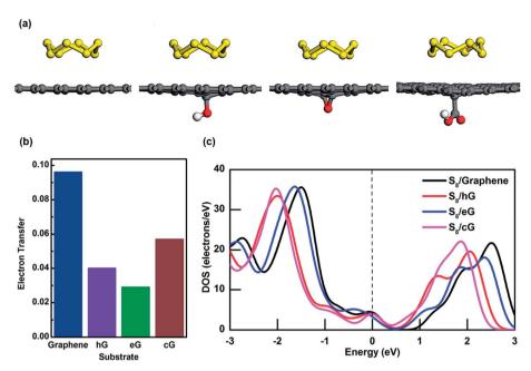
Fig. 4 (a)  $S_8$  adsorption on graphene, hG, eG and cG. Oxygen and hydrogen atoms are represented by red and white respectively. (b) Electron transfer from  $S_8$  to different substrates, and (c) density of states near Fermi energy region for  $S_8$  on graphene, hG, eG and cG.
