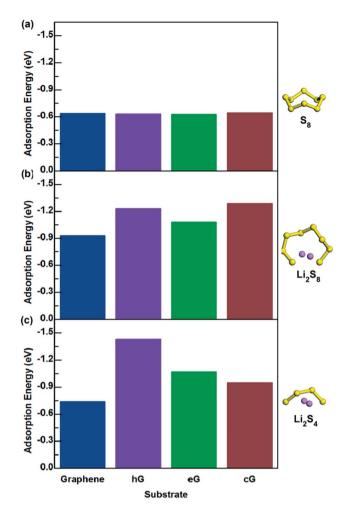
Fig. 3 Adsorption values of (a)  $S_8$ , (b)  $Li_2S_8$ , and (c)  $Li_2S_4$  interacting with graphene, hG, eG and cG.
