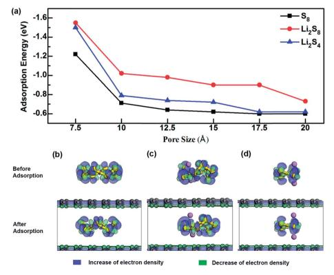
Fig. 2 (a) Adsorption energies of  $S_8$ ,  $Li_2S_8$  and  $Li_2S_4$  to microporous graphene. Deformation charge density and adsorption site of (b)  $S_8$ , (c)  $Li_2S_8$ , and (d) Li<sub>2</sub>S<sub>4</sub>.
