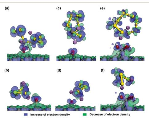
Fig. 6 Deformation charge density at Li<sub>2</sub>S<sub>8</sub> and Li<sub>2</sub>S<sub>4</sub> adsorption sites of (a and b) hG, (c and d) eG and (e and f) cG. (The increase/decrease of electron density is denoted by blue/green, respectively.)
