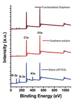
Fig. 4 (a) FTIR spectra of APTES, graphene solution (in water), and graphene functionalized with hydrolyzed APTES. (b) XPS survey spectra of APTES, pure graphene solution, and graphene solution functionalized with APTES.
