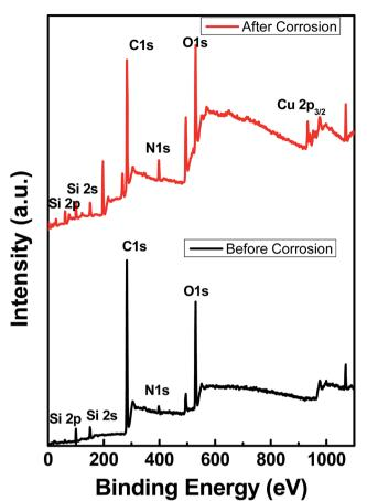
Fig. 7 XPS survey spectra of functionalized APTES before and after potentiodynamic polarization.
