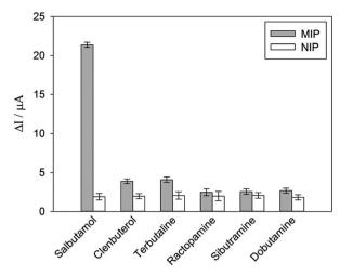
Fig. 5 DPV responses of MIP and NIP toward 1.2  $\mu$ M of salbutamol and other structurally related compounds.
