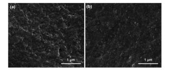
Fig. 2 SEM images of (a) MIP and (b) NIP modified graphene/PEDOT:PSS/SPCEs.
