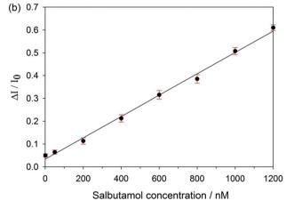
Fig. 3 (a) Differential pulse voltammograms of MIP/GP-PEDOT:PSS/SPCE recorded in 5 mM  $\rm K_3[Fe(CN)_6]/K_4[Fe(CN)_6]$  after incubation in different concentrations of salbutamol, (b) calibration curve of the MIP/GP-PEDOT:PSS/SPCE. The error bars represent the standard deviation obtained from 6 independent measurements.
