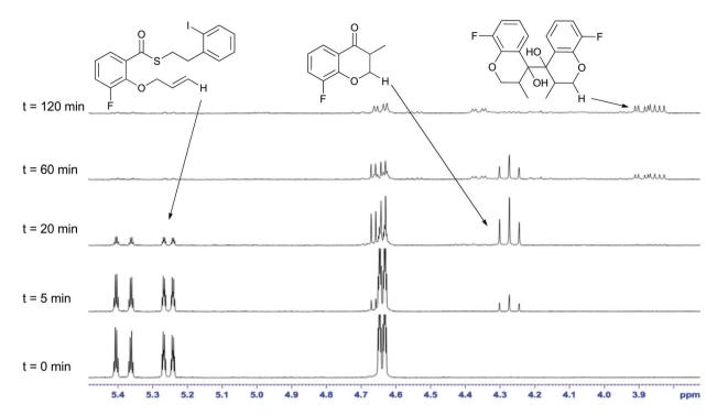
Fig. 1 In situ <sup>1</sup>H NMR analysis of the dimerization reaction mixture.
