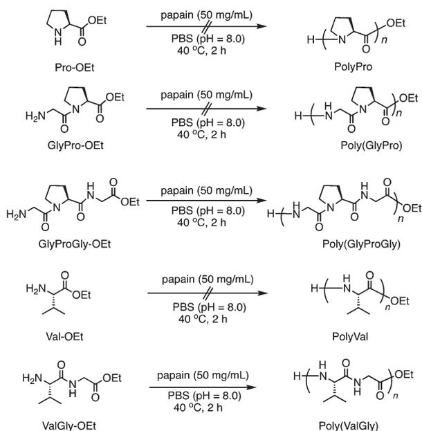
**Scheme 1** Chemoenzymatic polymerization of Pro- and Val-containing monomers using papain.
