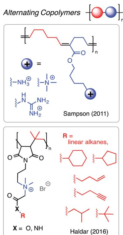
Fig. 17 Alternating copolymers as platforms for antibacterial polymers.
