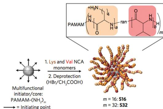
**Fig. 13** Antibacterial nanoparticles by ring-opening polymerization initiated by a PAMAM dendrimer core. This unique chain architecture influences the mechanism of activity relative to linear chains. Reproduced with permission from ref. 93, copyright 2016, Springer Nature.
