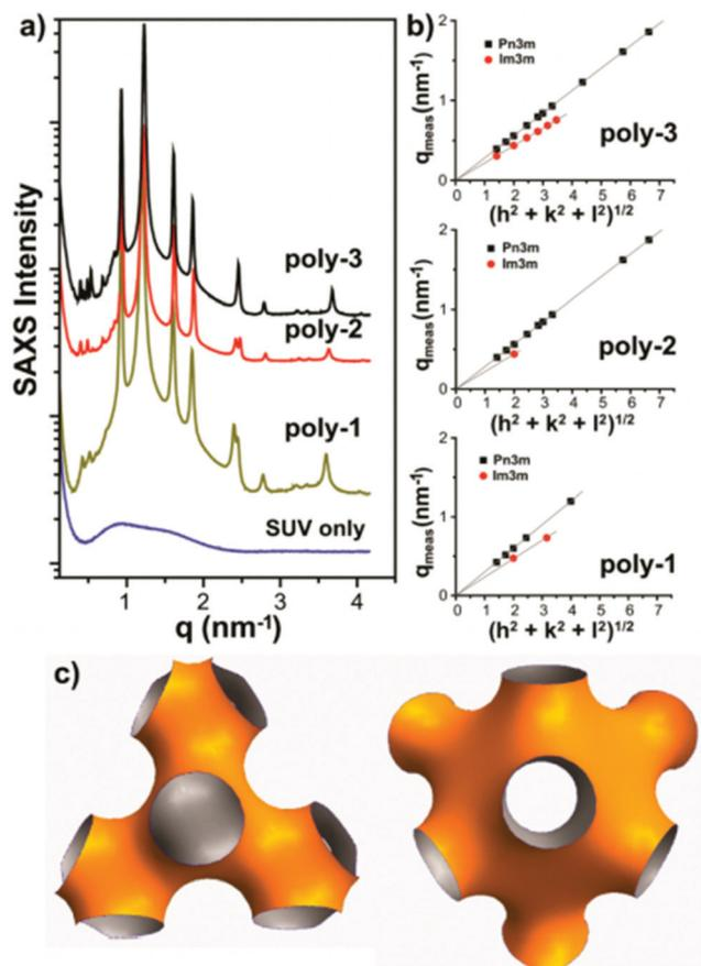
Fig. 21 SAXS data (a,b) for a lipid bilayer containing antimicrobial polymethacrylates and corresponding real space model (c). Reproduced with permission from ref. 157, copyright 2013, American Chemical Society.
