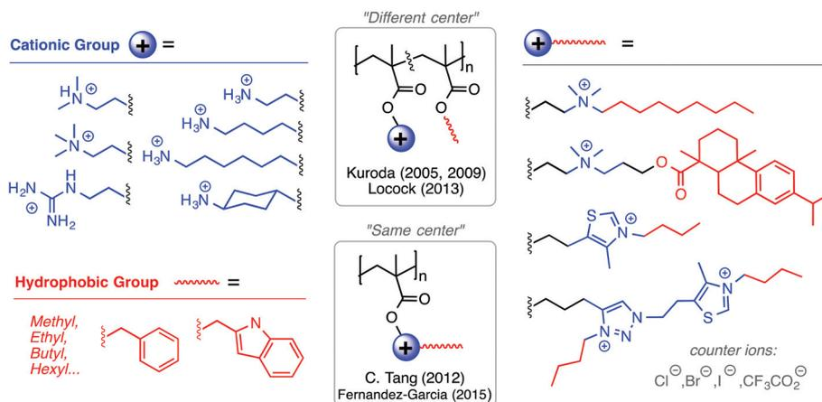
**Fig. 6** The broad diversity of cationic and hydrophobic group structures, and their relative spatial arrangements, have been extensively tailored in the poly(methacrylate) design platform towards the optimization of biological activity.
