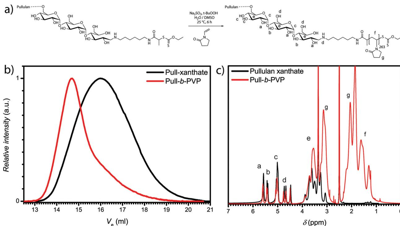
**Fig. 1** (a) Polymerization scheme for Pull-*b*-PVP block copolymer formation in water/DMSO mixture, (b) SEC traces of pullulan xanthate and Pull<sub>124</sub>-*b*-PVP<sub>263</sub> block copolymer synthesized in water/DMSO mixtures recorded in NMP at 70 °C and (c) <sup>1</sup>H-NMR of pullulan xanthate and Pull<sub>124</sub>-*b*-PVP<sub>263</sub> recorded at 400 MHz in DMSO-*d*<sub>6</sub>.
