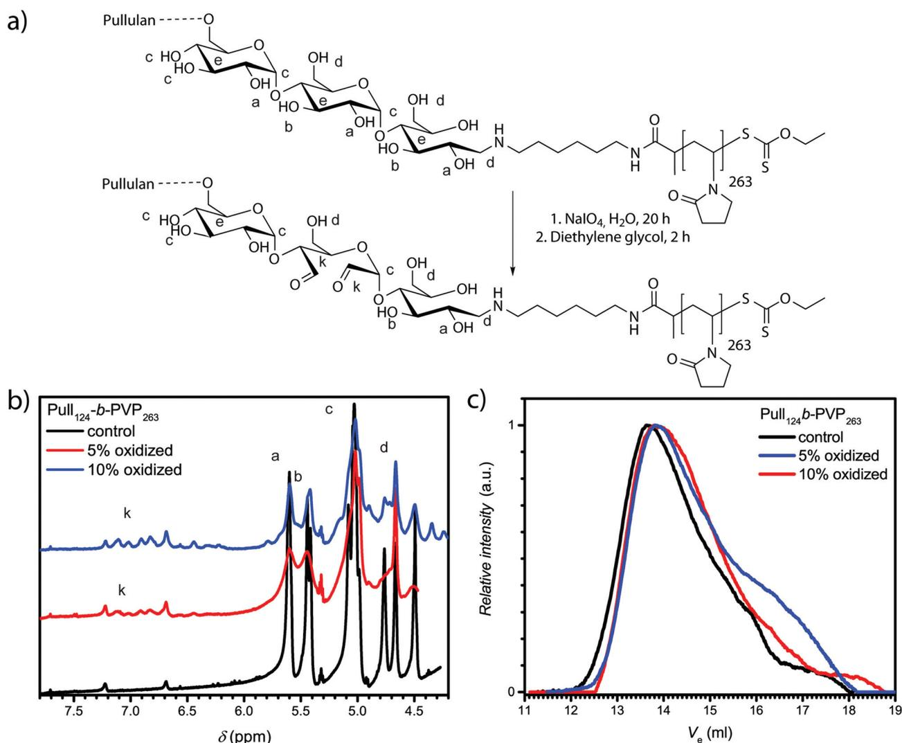
Fig. 3 (a) Schematic oxidation of Pull<sub>124</sub>-*b*-PVP<sub>263</sub> with NaIO<sub>4</sub>; (b) <sup>1</sup>H-NMR spectra of oxidized Pull<sub>124</sub>-*b*-PVP<sub>263</sub> emphasizing on the anomeric proton peaks of the oxidized glucose units recorded at 400 MHz in DMSO-*d*<sub>6</sub>; (c) corresponding SEC elution curves recorded in NMP at 70 °C.
