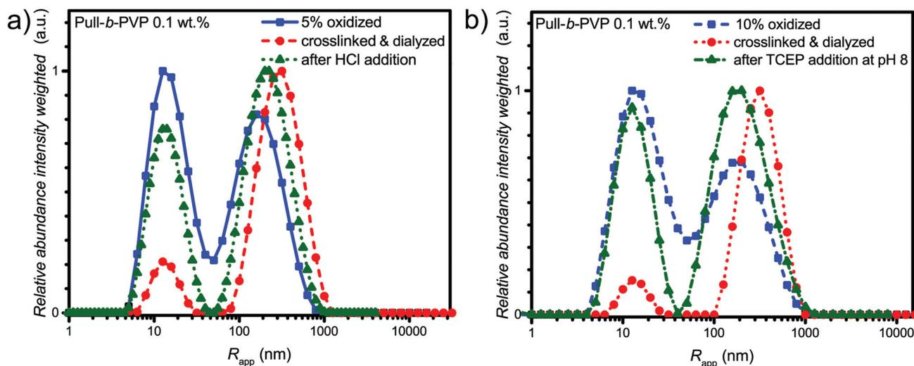
Fig. 5 Comparison of intensity weighted particle size distributions of 0.1 wt% solutions in Millipore water measured *via* DLS at 25 °C of (a) 5% oxidized Pull<sub>124</sub>-*b*-PVP<sub>263</sub>, oxidized block copolymer after crosslinking and dialysis and after treatment with HCl; (b) 10% oxidized Pull<sub>124</sub>-*b*-PVP<sub>263</sub>, oxidized block copolymer after crosslinking and dialysis and after treatment with TCEP.
