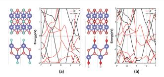
Fig. 6 (a and b) Side and top views of MnBX (X = F or OH) structural forms and the corresponding spin-polarized band structures.
