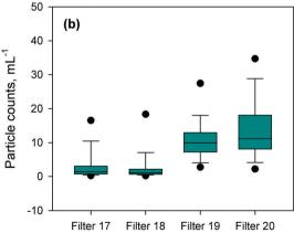
Fig. 1 Comparison of effluent (a) turbidity and (b) particle counts of the chlorinated anthracite filter and GAC biofilters. The boxes were generated from monthly average data from 2007–2017. The top and bottom of the boxes represent the 75th and 25th percentiles, the top and bottom whiskers represent the 90th and 10th percentiles, the black circles are the 5th and 95th percentiles, and the solid line in the box is the median. The target turbidity according to the US EPA's LT2 = 0.15 NTU.
