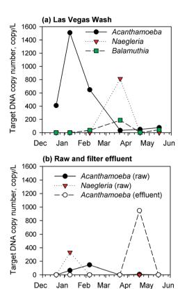
Fig. 3 Copy number concentrations of target DNA sequences of Acanthamoeba spp., Naegleria fowleri, and Balamuthia mandrillaris for samples collected from (a) the Las Vegas Wash and (b) the raw water from Lake Mead and GAC (i.e., filter 19) effluent from the RMWTF.
