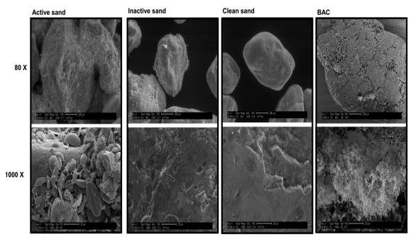
Fig. 1 SEM images of different media at 80× (top) and 1000× (bottom) magnification. From left to right, active sand, inactive sand, clean sand and biological activated carbon. Scale bars are 200  $\mu m$  for 80× and 20  $\mu m$  for 1000×.
