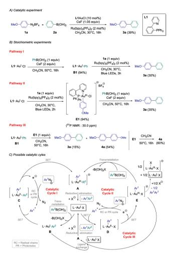
Scheme 2 Catalytic and stoichiometric experiments of the cross-coupling between 4-methoxybenzenediazonium tetrafluoroborate **1a** and phenylboronic acid **2a** using **L1**AuCl as the gold precursor, and possible catalytic cycles.
