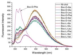
Fig. 2 Fluorescence changes of NI-chol 1 (10  $\mu$ M) in CH<sub>3</sub>CN-DMSO (95:5, v/v) with  $\square$  and  $\bot$  isomers of Ala, Glu, Leu, Phe, Ser and Val (500  $\mu$ M).  $(\lambda_{ex} = 325 \text{ nm, slit } 3 \times 5).$
