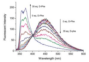
Fig. 3 Fluorescence based titrations of NI-chol 1 (10 μM) in CH<sub>3</sub>CN-DMSO (95:5, v/v) with various equivalents of Boc-D-Phe.
