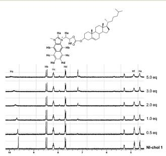
Fig. 5 Partial  $^{1}$ H NMR spectra (300 MHz) of **NI-chol 1** (5 mM) upon the addition of Boc-D-Phe (tetrabutylammonium salt) in CD<sub>3</sub>CN-DMSO- $d_6$  (95:5, v/v).
