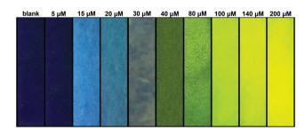
Fig. 4 Photograph showing the colour changes of **TCBT-OMe** impregnated test strips after addition to water samples containing different concentrations of HClO/ClO<sup>-</sup> under UV light (365 nm).
