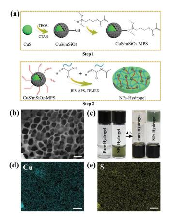
Fig. 1 (a) Schematic illustration of the synthetic route of CuS/mSiO<sub>2</sub>-MPS/poly(NIAAm-co-AAm) hydrogel. (b) SEM image of the dispersed CuS NPs in NPs-Hydrogel derived from radical polymerization. Scale bar, 5  $\mu m$ . (c) Photographs of the sol and gel states before or after radical polymerization for 4 h. (d, e) EDS elemental maps (Cu in green, S in yellow) of the NPs-Hydrogel. Scale bar, 5  $\mu$ m.
