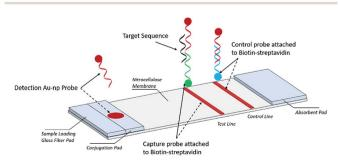
Fig. 1 Schematic depicting the lateral flow assay.
