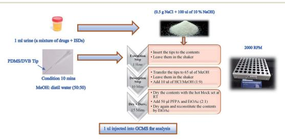
Fig. 1 Illustration of the optimum condition procedure applied to SPME PDMS/DVB fibre tips in the mixture of drugs in urine samples.
