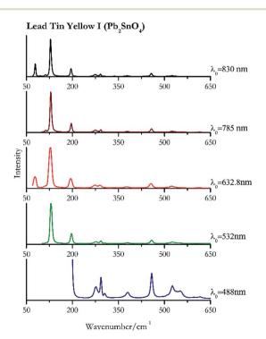
Fig. 19 Raman spectra of lead tin yellow I.
