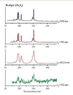
Fig. 7 Raman spectra of realgar.
