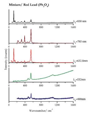
Fig. 1 Raman spectra of minium or red lead.
