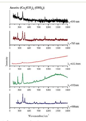
Fig. 15 Raman spectra of azurite.
