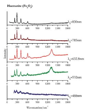
Fig. 2 Raman spectra of haematite.
