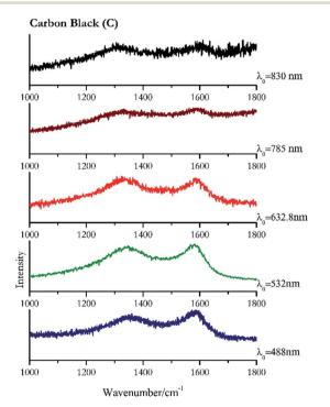
Fig. 25 Raman spectra of carbon black.
