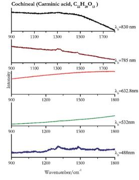
Fig. 8 Raman spectra of cochineal.
