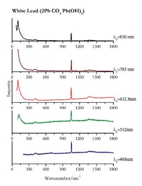
Fig. 22 Raman spectra of white lead.
