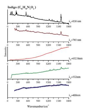
Fig. 14 Raman spectra of indigo.
