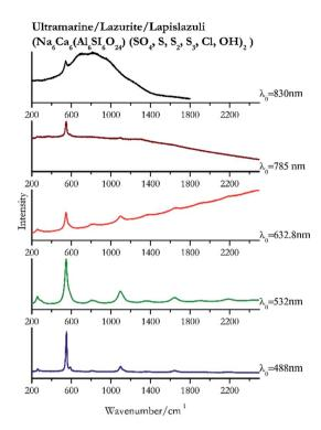
Fig. 16 Raman spectra of ultramarine.
