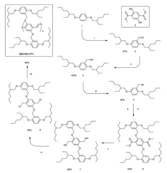
Scheme 1 The synthesis of the polymer BBEHBO-PPV. Reagents and conditions: (i) BuLi, TMEDA, hexane, then DMF; (ii) NaBH<sub>4</sub>, methanol; (iii) CBr<sub>4</sub>, (C<sub>6</sub>H<sub>5</sub>)<sub>3</sub>P, THF; (iv) K<sub>2</sub>CO<sub>3</sub>, DMF, 80 °C, 3 days; (v) LiAlH<sub>4</sub>, THF; (vi) (C<sub>6</sub>H<sub>5</sub>)<sub>3</sub>P, CCl<sub>4</sub>, M<sub>W</sub> 120 °C, 2 hours; (vii) tert-BuOK, THF
