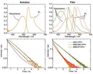
Fig. 1 Top: Absorption and PL spectra of BBEHBO-PPV in solution at  $0.025 \ \text{mg ml}^{-1}$  (top left) and as a film (top right). The absorption and PL spectra of MEH-PPV and BBEHP-PPV as films are also shown top right. Bottom: Photoluminescence lifetime measurements in solution (bottom left) and film (bottom right) for BBEHP-PPV, MEH-PPV and BBEHBO-PPV.
