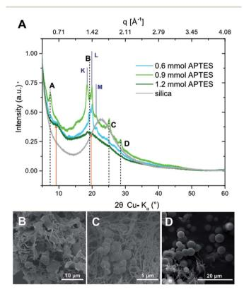
Fig. 6 PI6/SiO<sub>2</sub> prepared from PMA, HMDA, APTES and TEOS. (A) Diffractograms of the hybrids prepared at different  $n_{APTES}$ , and diffractogram of hydrothermally synthesized  $SiO_2$  for comparison (gray). (B)–(D) SEM images of the corresponding hybrids at  $n_{APTES} = 0.6$  mmol (B),  $n_{APTES} = 0.9$  mmol, and  $n_{APTES} = 1.2$  mmol.
