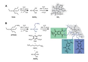
Fig. 4 Reaction equation of  $SiO_2$  and  $PI6/SiO_2$  co-condensation. (A) Hydrothermal hydrolysis and condensation sequence from TEOS to  $SiO_2$ . (B) Co-condensation of PI6 and  $SiO_2$  in the presence of the compatibilizer APTES; possible linkages (1,2-diamide, amic acid; and imide) are shown.
