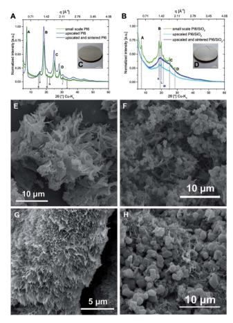
Fig. 7 Pl6 and Pl6/SiO<sub>2</sub> upscaling and sintering. (A) and (B) Comparison of the diffractograms of small scale synthesis, upscaled synthesis and material after sintering (Pl6: (A) Pl6/SiO<sub>2</sub>: (B)). (C) and (D) Photographs of the Pl6 (C), and the Pl6/SiO<sub>2</sub> pellet from sintering. (E)–(H) SEM images of upscaled Pl6 before (E) and after (G) sintering, and of upscaled Pl6/SiO<sub>2</sub> before (F) and after (H) sintering.
