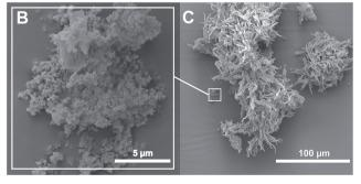
Fig. 5 Pl6/SiO<sub>2</sub> hybrids prepared from HMDA, PMA and TEOS. (A) Diffractograms of Pl6/SiO<sub>2</sub> prepared using different  $n_{\rm TEOS}$ ; amorphous backgrounds are highlighted. (B) and (C) SEM images of Pl6/SiO<sub>2</sub> at  $n_{\rm TEOS}=1.5$  mmol; SiO<sub>2</sub> nanoparticles (B) coexist with Pl6 ribbons (C).
