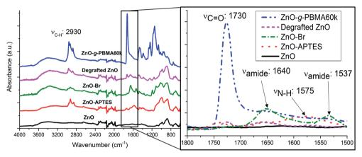
Fig. 2 FTIR spectra of ZnO, ZnO-APTES, ZnO-Br, ZnO-g-PBMA60k and degrafted ZnO between 4000 and 600 cm $^{-1}$ . Spectra have been vertically scaled and offset for clarity. The enlarged spectrum shows detailed overlapping spectra between 1800 and 1500 cm $^{-1}$  without offset.
