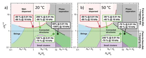
Fig. 13 The relative loss tangent as a percentage at 0.01 Hz and 10 kHz for the nanocomposites with grafted NPs at 20 °C (a) and 50 °C (b).
