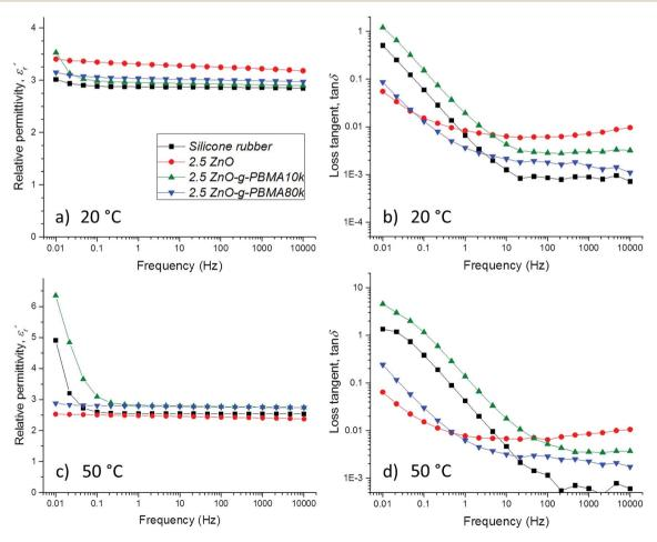
Fig. 12 Dielectric spectroscopy data of silicone rubber, 2.5ZnO, 2.5ZnO-g-PBMA10k and 2.5ZnO-g-PBMA80k at 20 °C (a and b), and 50 °C (c and d). Fig. (a) and (c) display the relative permittivity,  $\varepsilon'_r$  versus frequency, and (b) and (d) the loss tangent, tan  $\delta$  versus frequency.
