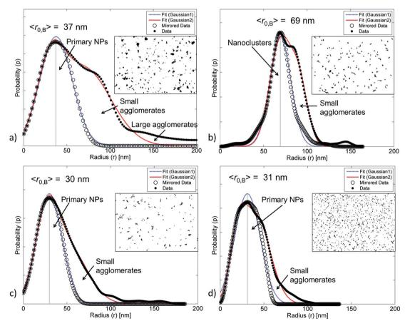
Fig. 5 The size distribution and the mean radius calculated from transmission images of (a) ZnO NPs, (b) ZnO-APTES, (c) ZnO-g-PBMA10k and (d) ZnO-g-PBMA80k. The arrows show the areas under the curves, representing the fraction of primary NPs, small and large agglomerates. The inset images are 12  $\mu$ m wide cut-outs of the full images for simplified comparison.
