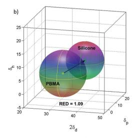
Fig. 6 (a) Hansen's solubility parameters for ZnO in silicone resin give RED = 0.41 indicating compatibility. (b) HSPs for PBMA in silicone resin indicate semi-compatibility as RED = 1.09.
