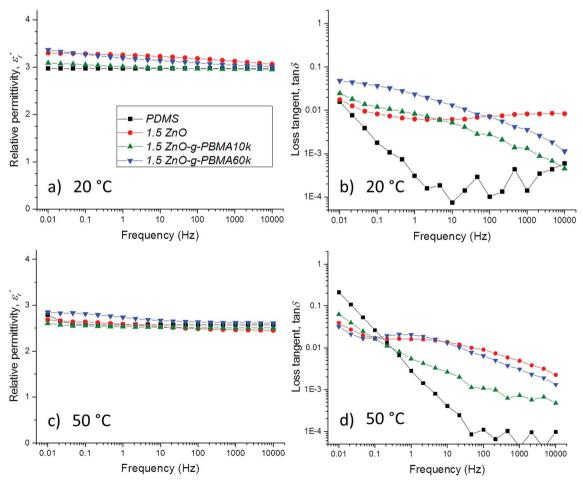
Fig. 11 Dielectric spectroscopy data of neat *PDMS*, 1.5ZnO, 1.5ZnO-g-PBMA10k and 1.5ZnO-g-PBMA60k at 20 °C (a and b) and at 50 °C (c and d). Fig. (a) and (c) show the relative permittivity,  $\varepsilon'_r$  versus frequency, and (b) and (d) the loss tangent,  $\tan \delta$  versus frequency.
