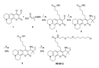
Scheme 5 Synthesis of RFAP-2. Reagents and conditions: (i) Pd-PEPPSI-IPr, K<sub>3</sub>PO<sub>4</sub>·H<sub>2</sub>O, THF, rt, 10 h; (ii) NH<sub>3</sub>, MeOH, 0 °C, then prenylboronic acid, rt, 10 h; (iii) LiOH, THF/MeOH/H2O, rt, 6 h; (iv) 2-(2-((6-chlorohexyl)oxy)ethoxy)ethan-1-amine, HATU, DIPEA, DMF, rt, 12 h.
