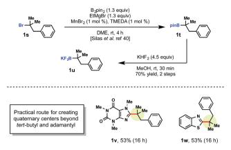
Scheme 4 Synthesis of tertiary alkyltrifluoroborate<sup>a</sup>. <sup>a</sup>Reactions were run with heteroarene (1.0 equiv.), tertiary alkyltrifluoroborate (1.0 equiv.), MesAcr (5 mol%), K<sub>2</sub>S<sub>2</sub>O<sub>8</sub> (2.0 equiv.), trifluoroacetic acid (1.0 equiv.) in MeCN/H2O (1:1) on 0.3 mmol scale.
