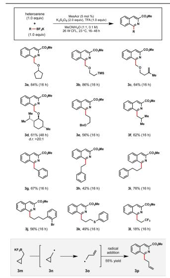
$<sup>^</sup>a$  Reactions were run with 1-methyl isoquinolinecarboxylate (1.0 equiv.), primary alkyltrifluoroborate (1.0 equiv.), MesAcr (5 mol%),  $\rm K_2S_2O_8$  (2.0 equiv.), trifluoroacetic acid (1.0 equiv.) in MeCN/H<sub>2</sub>O (1:1) on 0.3 mmol scale.
