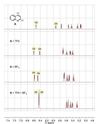
Fig. 2  $\,^{1}$ H NMR of A with trifluoroacetic acid and/or BF $_{3}$  additive in CD $_{3}$ CN/H $_{2}$ O (1 : 1). TMS was used as a reference.
