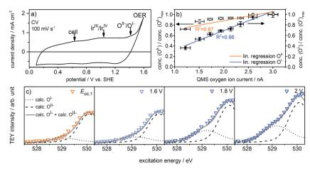
Fig. 2 (a) Cyclic voltammogram, (b) normalized  $O^{1-}$  and  $O^{1-}$  concentrations over QMS oxygen ion current, and (c) zoomed and fitted low excitation energy regions of O K-edges recorded in the three-electrode cell (indicated potentials vs. SHE, ring current = 60 mA, p = 0.3 Pa, 0.1 M  $H_2SO_4$ ).
