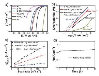
Fig. 3 HER tests in 1 M KOH. (a) The HER polarization plots for different catalysts at a scan rate of 5 mV s<sup>-1</sup>. (b) Tafel plots and exchange currents for different catalysts. (c) The capacitive currents at different scan rates. The mass loading is 0.50 mg cm<sup>-2</sup> supported on a glassy carbon (GC) electrode for the tests in (a–c). (d) The stability test for Ni/Mo<sub>2</sub>C-PC on Ni foam with a loading of 2 mg cm<sup>-2</sup>.
