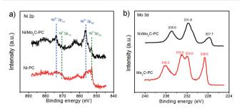
Fig. 4 (a) High-resolution Ni 2p XPS spectra for Ni/Mo $_2$ C-PC and Ni-PC. (b) High-resolution Mo 3d XPS spectra for Ni/Mo $_2$ C-PC and Mo $_2$ C-PC.
