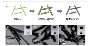
Fig. 1 (a) Illustration of the synthesis of Ni/Mo<sub>2</sub>C-PC from NiMoO<sub>4</sub> nanorods. (b-d) TEM images of (b) NiMoO<sub>4</sub>, (c) NiMoO<sub>4</sub>@PDA, and (d) Ni/Mo<sub>2</sub>C-PC. Insets are the corresponding digital photographs.
