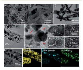
Fig. 2 (a) Low and (b) high magnification SEM images of Ni/Mo<sub>2</sub>C-PC. (c) Low and (d and e) high magnification TEM images of Ni/Mo<sub>2</sub>C-PC; the arrows in (e) show the porosity. (f and g) HRTEM images of (f) Ni and (g) Mo<sub>2</sub>C. (h) EELS elemental mapping images of C, Mo, and Ni.
