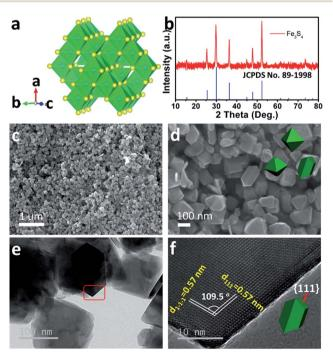
Fig. 1 Structure characterization of the as-prepared  $Fe_3S_4$ . (a) Crystal structure and (b) XRD pattern of the as-prepared  $Fe_3S_4$ . (c and d) SEM images, (e) TEM and (f) HRTEM images for the as-prepared  $Fe_3S_4$ .
