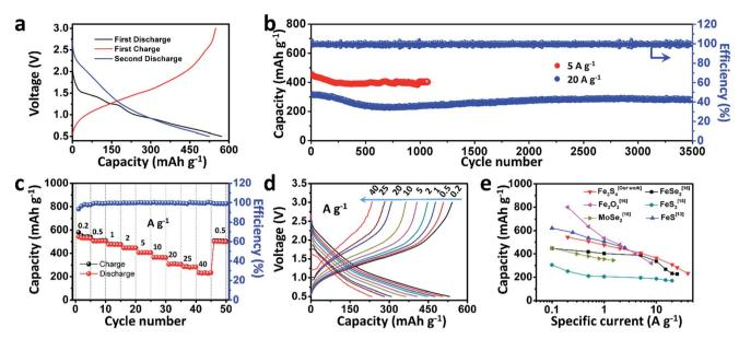
Fig. 2 Electrochemical performance of the as-prepared  $Fe_3S_4$ . (a) Discharge-charge curves of the first two cycles at a specific current of 0.2 A  $g^{-1}$ ; (b) cycling performances at 5 and 20 A  $g^{-1}$ ; (c) rate capability and (d) discharge-charge curves at various current rates; (e) comparison of the as-prepared  $Fe_3S_4$  with other conversion anode materials of SIBs.
