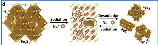
Fig. 4 (a) TEM image, (b) SAED pattern and (c) HRTEM image of the as-prepared  $Fe_3S_4$  at a full charge state after 200 cycles. (d) Schematic illustration of the sodium-storage mechanism in the  $Fe_3S_4$  electrode.
