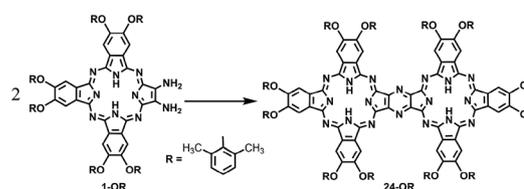
**Scheme 1** Schematic showing the synthesis of the metal-free homobinuclear phthalocyanine 24-OR in CH<sub>2</sub>Cl<sub>2</sub> at room temperature in the mixed solvent of CH<sub>2</sub>Cl<sub>2</sub> and TFA (in the ratio of 80 : 20), with 1-OR as the starting reagent.
