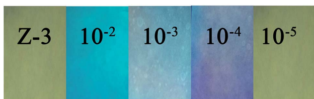
Fig. 5 Photographs of test strips (the concentration of \text{Hg}^{2+} is 0 M, 10^{-1} M, 10^{-2} M, 10^{-3} M, 10^{-4} M, 10^{-5} M, both under an UV lamp at 365 nm).
