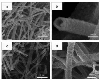
Fig. 20 (a) Low- and (b) high-magnification SEM images of  $\text{In}_2\text{O}_3$  and (c) low- and (d) high-magnification SEM images of  $\text{Fe}_2\text{O}_3\text{-In}_2\text{O}_3$  nanotubes after annealing at  $500\text{ }^\circ\text{C}$  (this figure has been adapted from ref. 73 with permission from Elsevier).
