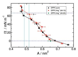
Fig. 2 Surface-pressure/area isotherms at 310 K for a DPPC monolayer on pure water (black points), and on an aqueous solution of ArgCl with a DPPC: Arg+ ratio of 64:10 (red points). The green dot corresponds to a DPPC: Arg<sup>+</sup> ratio of 64: 20. The region of coexistence between the liquid-expanded and liquid-condensed phases is highlighted by the cyan vertical lines.
