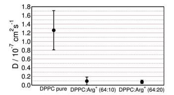
Fig. 6 DPPC self-diffusion coefficients computed for the monolayer on pure water, and the 64 : 10 and 64 : 20 DPPC : Arg $^+$  systems, at  $\it II$   $\sim$  1 mN m $^{-1}$ .
