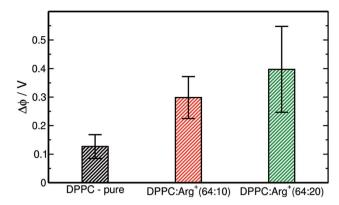
Fig. 4 Surface potential of the DPPC monolayer on pure water (black), and the 64 : 10 (red) and 64 : 20 (green) DPPC : Arg $^+$  systems, at  $\it H \sim 1$  mN m $^{-1}$ . The potential values are:  $\Delta\phi_{\rm DPPC}=0.13\pm0.04$  V,  $\Delta\phi_{64:10}=0.30\pm0.07$  V,  $\Delta\phi_{64:20}=0.40\pm0.15$  V.
