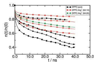
Fig. 7 Cage correlation function, n(t), for different systems at various surface pressures. Black lines = DPPC monolayer on pure water, red lines = 64 : 10 DPPC : Arg<sup>+</sup> system, green line = 64 : 20 DPPC : Arg<sup>+</sup> system. Circles:  $II \sim 70$  mN m $^{-1}$ ; diamonds:  $II \sim 50$  mN m $^{-1}$ , triangles:  $II \sim 20$  mN m $^{-1}$ , and squares:  $II \sim 1$  mN m $^{-1}$ .
