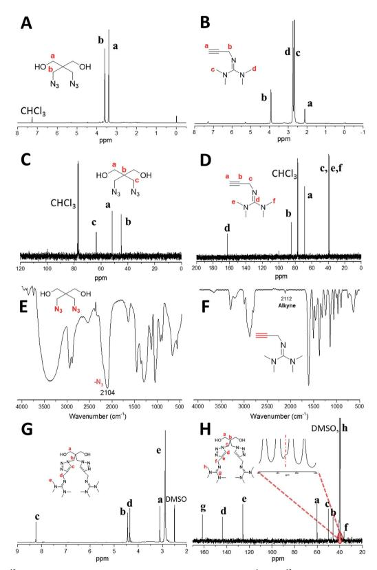
Fig. 2  $^{1}$ H NMR,  $^{13}$ C NMR and FT-IR spectra of DAzD (A, C and E), TMG-Al (B, D and F) and  $^{1}$ H NMR,  $^{13}$ C NMR spectra of TMG-OH (G and H) in CDCl<sub>3</sub> or DMSO- $d_6$ .
