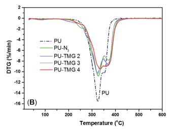
Fig. 7 TGA (A) and DTG (B) curves of PU, PU-N<sub>3</sub>, PU-TMG 2 (wt% = 1.0%), PU-TMG 3 (wt% = 2.1%), and PU-TMG 4 (wt% = 5.5%) under nitrogen.
