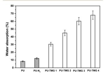
Fig. 8 Water absorption properties of PU, PU-N<sub>3</sub>, PU-TMG 1 (wt% = 0.6%), PU-TMG 2 (wt% = 1.0%), PU-TMG 3 (wt% = 2.1%), and PU-TMG 4 (wt% = 5.5%) at room temperature for 72 hours.
