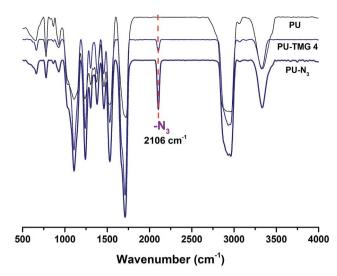
Fig. 4 FT-IR spectra of polyurethane (PU), click-suitable polyurethane (PU- $N_3$ ) and polyurethane with side-chain tetramethylgermanium (PU-TMG 4).
