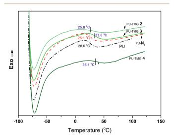
Fig. 6 DSC curves of PU, PU-N $_3$ , PU-TMG 2 (wt% = 1.0%), PU-TMG 3 (wt% = 2.1%), and PU-TMG 4 (wt% = 5.5%).
