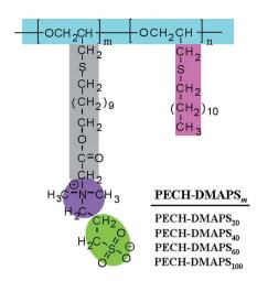
Fig. 1 Chemical structures of the PECH-DMAPS<sub>m</sub> polymers used in this study
