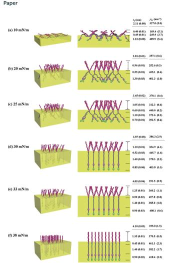
Fig. 9 Molecular models of the Langmuir films of PECH-DMAPS $_{60}$  prepared at the air–water interface under various surface pressures: (left) view with a tilt angle from the top; (right) front view along the polymer backbone.
