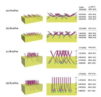
Fig. 7 Molecular models of the Langmuir films of PECH-DMAPS $_{20}$  prepared at the air-water interface under various surface pressures: (left) view with a tilt angle from the top; (right) front view along the polymer backbone.
