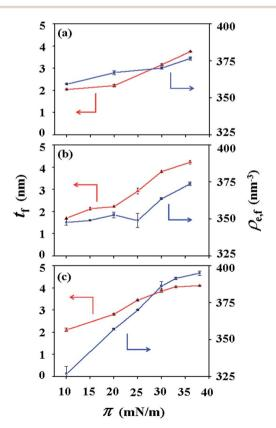
Fig. 5 Thickness  $t_{\rm f}$  and electron density  $\rho_{\rm e,f}$  variations of the Langmuir film prepared on the air–water interface as a function of surface pressure: (a) PECH-DMAPS<sub>20</sub>; (b) PECH-DMAPS<sub>40</sub>; (c) PECH-DMAPS<sub>60</sub>.
