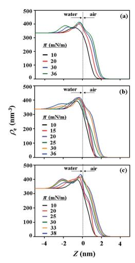
Fig. 6 Electron density  $\rho_{\rm e}$  profiles as a function of the film thickness, for the films prepared at the air–water interface under various surface pressures: (a) PECH-DMAPS<sub>20</sub>; (b) PECH-DMAPS<sub>40</sub>; (c) PECH-DMAPS<sub>60</sub>.
